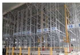
堆垛机立库 ASRS with Stack Crane
