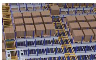
同巷道多车协同作业 Multi shuttle cooperative operation in the same roadway
